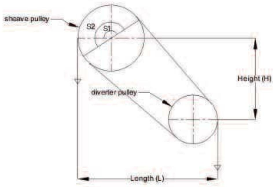
Figure 4: Double-wrap traction
