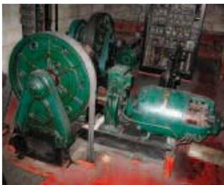
Figure 3: SWT (angle of contact: 180°)
