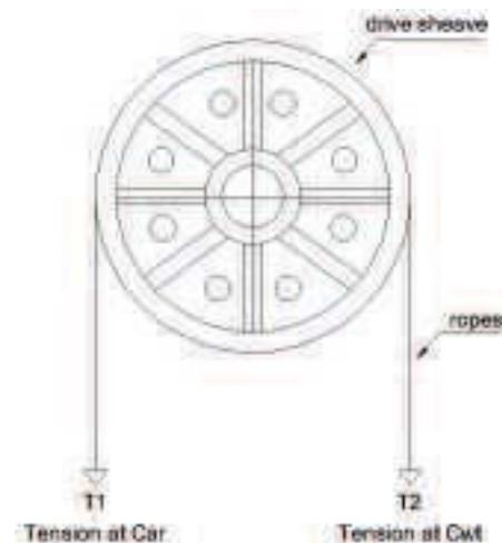
Figure 2: Traction calculation
